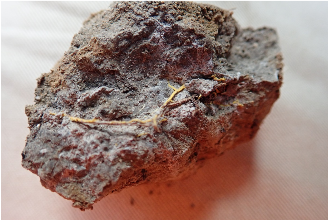
Figure 26. A tree root of Coatesia paniculata recorded at 6.1mbgl in BH6 with distinctive yellow colouration.
